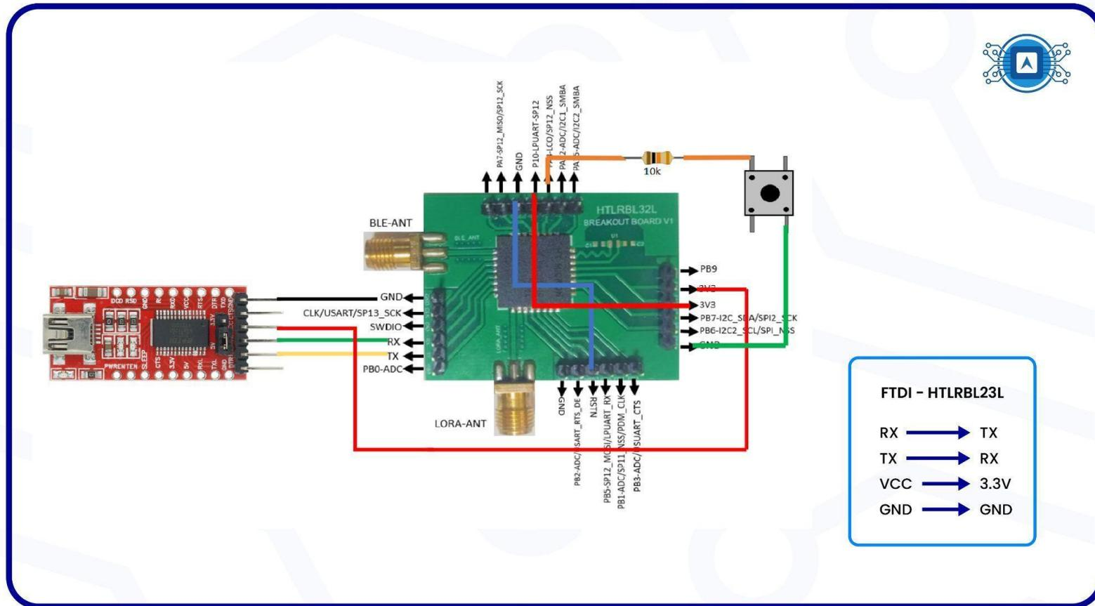
Image 1: Electronic schematic of the board. Source: *The author.*
