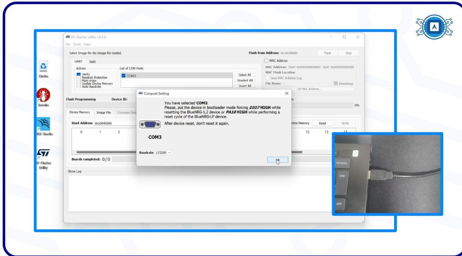
Image 3: Connecting the board to the computer through UART(FTDI). Source: *The author*.
