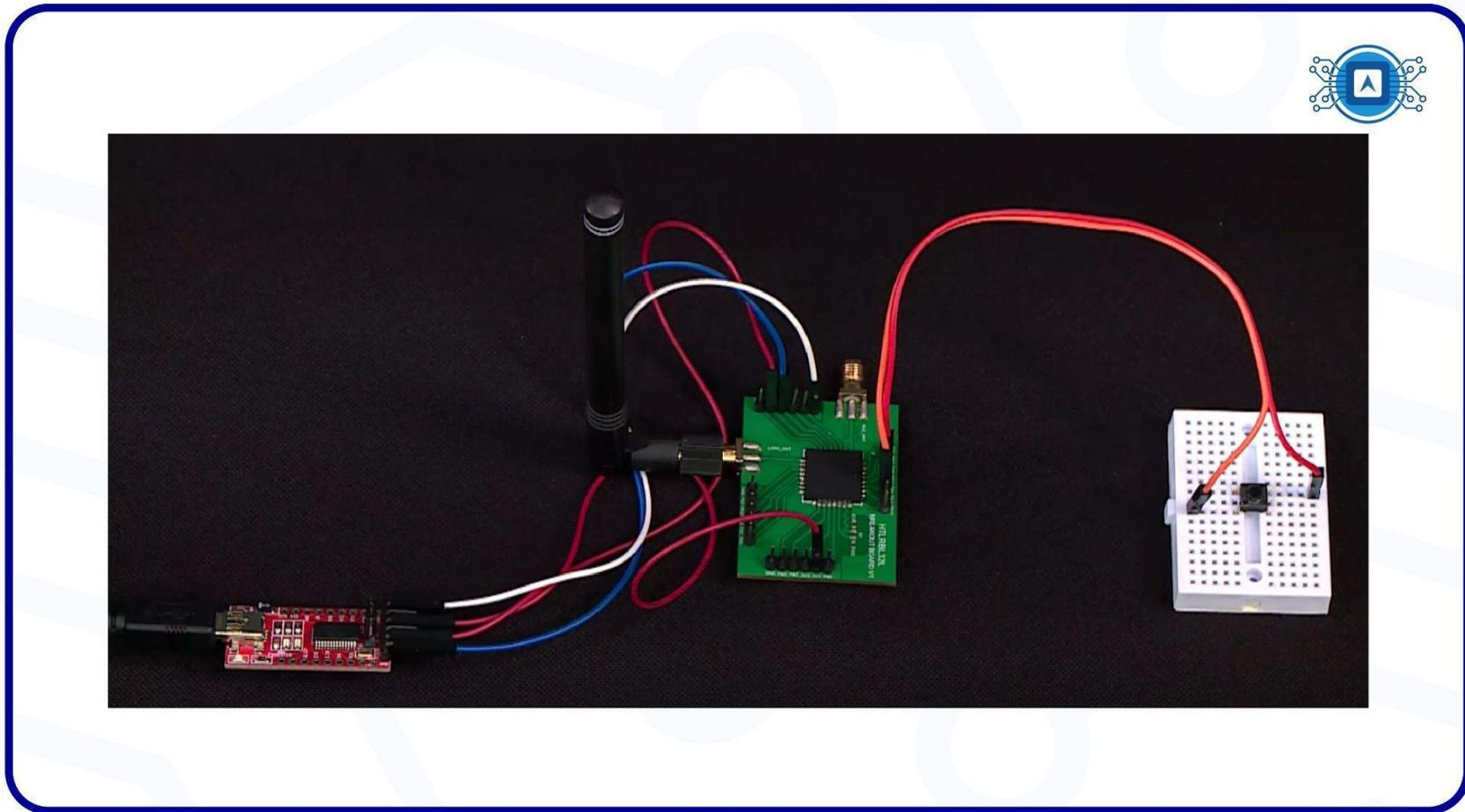
Image 2: Plate physically assembled according to the electronic schematic. Source: *The author*.
