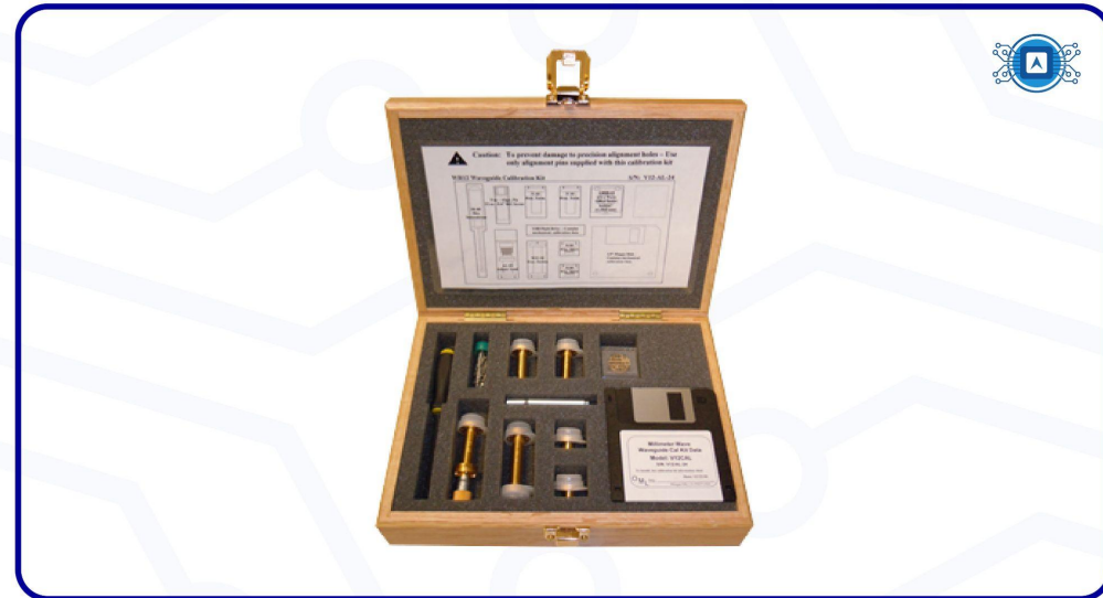
Image 08: Box with coaxial calibration kit. Source: Omlink < https://www.omlinc.com/22-products/vna-calibration-kit/7-vna-calibration-kit >.
